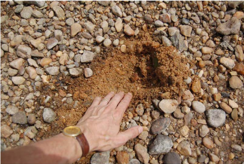
Figure 11. Single layer of armor gravel overlying a mix of coarse sands and gravels at the upper bar.
